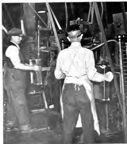
A worker in the factory showing a battery of spot welders working on drawer casings.
